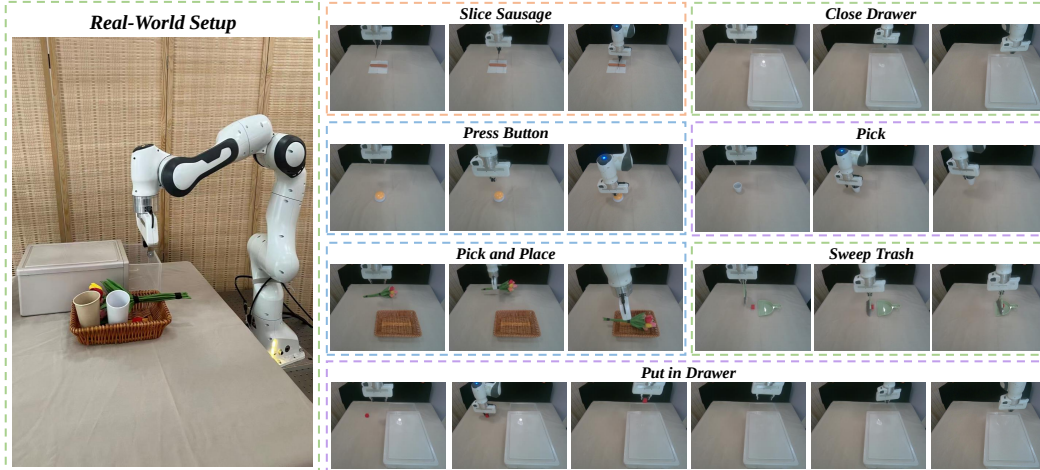
Figure 5: Real-world Setup and Task Execution. (Left) Real-robot evaluation environment; (Right) Visualizations of our policy executing manipulation tasks.
